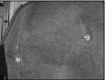
**STEP 5** Place the rear factory clip back into place.
